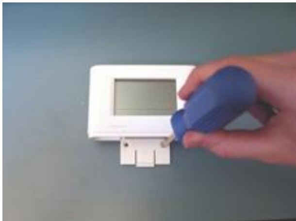
Illustration: Mounting the HUMLOG 10
