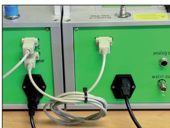
Establish a serial connection between the automatic calibration module and the PC/notebook.
