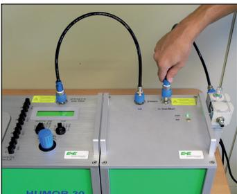
Attach the oil separator to the side of the automatic calibration module, on the bracket, and establish a connection to the input "Pressure in".
