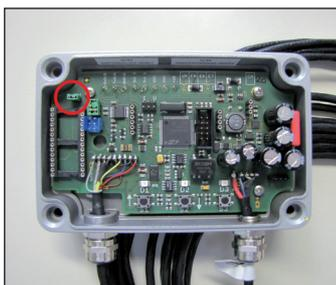
5. Connect the test unit to the supply connections of HUMOR 20.
