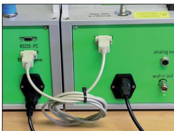
Establish a serial connection between HUMOR 20 and the automatic calibration module. Connect "RS232-Humor" on the automatic calibration module with "RS232" on HUMOR 20. (Max. cable length allowed is 3m. The length of the supplied cable is 1.8m)
