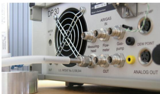
3. Connect the flow meter to the gas outlet of the chilled mirror dew point meter.
