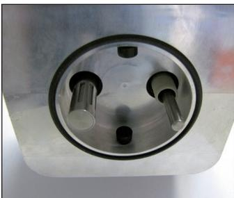
1. Plug both air vents of the cover of the measurement chamber with the plugs supplied with the adapter (see left picture).
