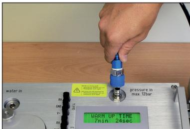
8. The 6th adjustment point is set at 100% RH. Therefore disconnect HUMOR 20 from the compressed air supply.
